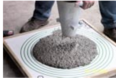
Slump Flow of SCC Mix
