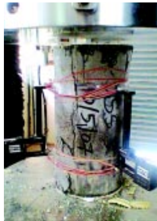
Crushing of Fibred RPC Cylinder without Spalling
