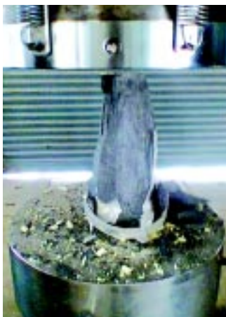
Spalling of Plain RPC Cylinder after failure
