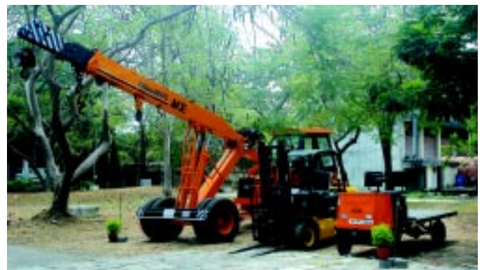
Hydraulic mobile crane of 11 ton capacity procured at SERC
